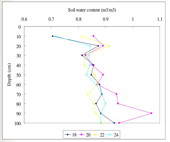
Values of more than 1 (100%) in volumetric water content indicates that the general conversion equation described in the user manual for the Profile Probe can not be applied to this peat .
