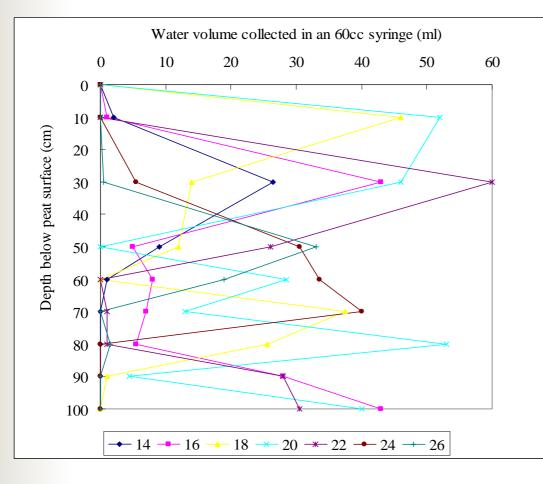
Depth variations in water volume in MGC were extremely wider compared to depth variations in Profile Probe outputs.
