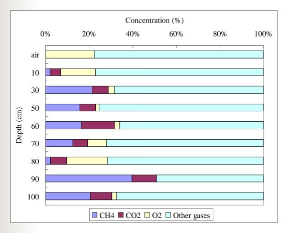
Water Table Level: 6.6cm Ground Vegetation: Sphagnum spp. Carex spp. Shrub Vegetation: none Although water table was fairly high level, methane was far less detected compared to other locations.
